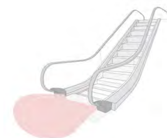
Figure 10-44: Example of Pedestrian Detection Method Using Motion Sensors
