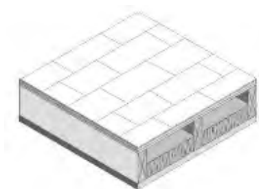
Figure 22: 5th: Wood Frame Rafter Roof (2022 Ref. App. Fig. 4.2.2)
