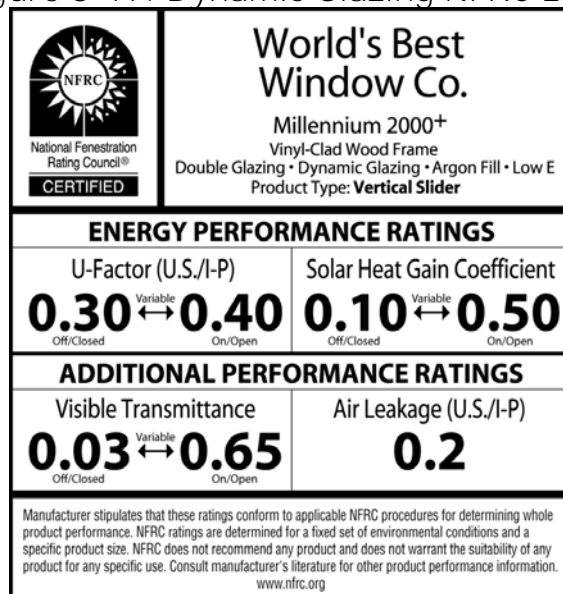
Figure 3-17: Dynamic Glazing NFRC Label
