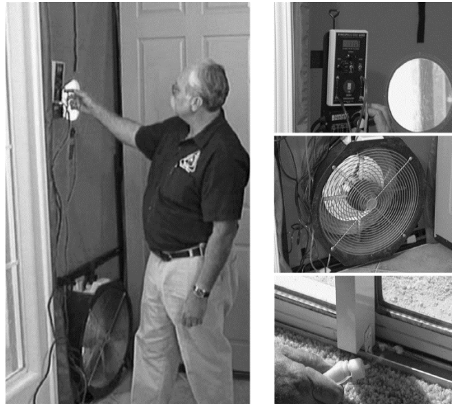
Figure 3-52: Blower Door Testing
