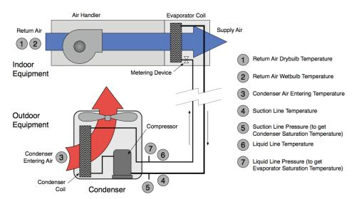
Figure 4-45: Measurements for Refrigerant Charge and Airflow Tests
