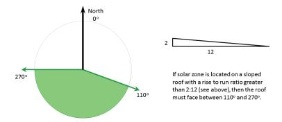
If a solar zone is located on a low-sloped roof (ratio of rise to run of 2:12 or less), the orientation requirement does not apply.
