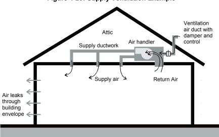
Figure 4-29: Supply Ventilation Example
