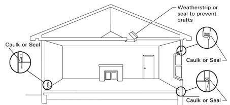
Figure 3-9: Caulking and Weatherstripping
