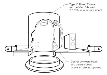
Figure 3-14: IC-Rated Luminaire (Light Fixture)
