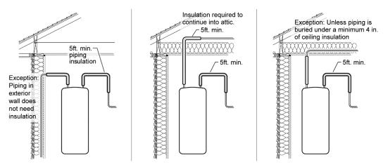
Table 5-7: Pipe Insulation Thickness Requirement (Excerpt From Table 120.3-A of the Energy Standards)
