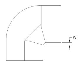
Figure 5-16: Measuring "w" at the Pool Site
