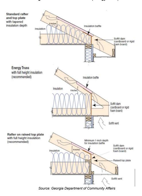
Figure 3-40: Raised Heel Truss (Energy Truss)
