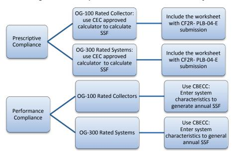
Figure 5-14: Compliance Process for Solar Thermal System
