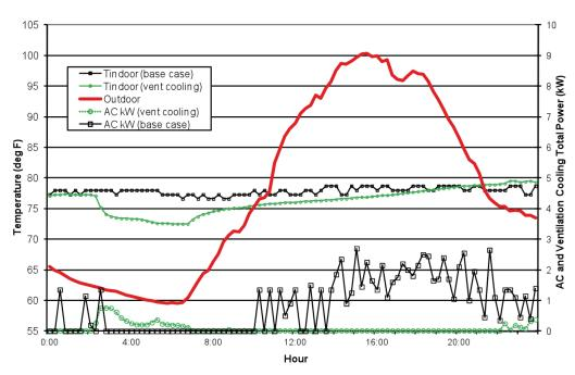
Figure 4-36: Diurnal Temperature Variation and Ventilation Cooling
