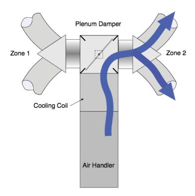
This diagram shows a common two-zone, single-damper system with zone 2 open (i.e., only zone 2 is calling for cooling).
