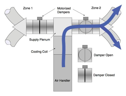
This diagram shows a common two-zone, two-damper system with zone 2 open (i.e., only zone 2 is calling for cooling).
