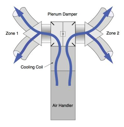
This diagram shows a common two-zone, single-damper system with both zones open (i.e., both zones are calling for cooling).
