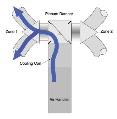
This diagram shows a common two-zone, single-damper system with zone 1 open (i.e., only zone 1 is calling for cooling).
