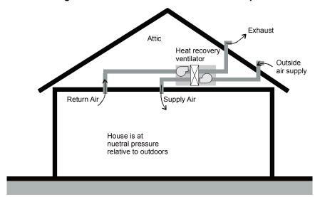
Figure 4-30: Combination Ventilation Example
