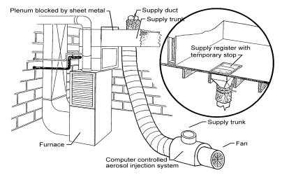
Figure 4-26: Computer-Controlled Aerosol Injection System
