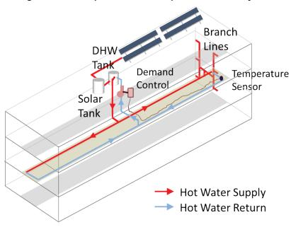
Figure 5-6: Example of a Dual-Loop Recirculation System
