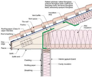
Figure 31: Vented Attic – Tile Roof – Air Permeable Insulation On Underside of Roof Deck - Can be
