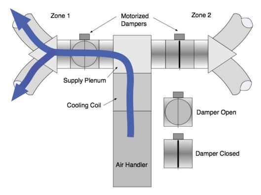
This diagram shows a common two-zone, two-damper system with zone 1 open (i.e., only zone 1 is calling for cooling).
