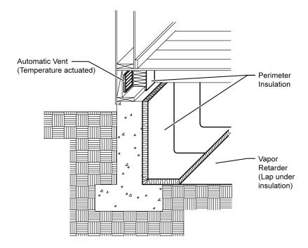
Figure 3-45: Controlled Ventilation Crawl Space
