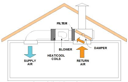
Figure 4-41: Central Fan System (Return Air Mode)
