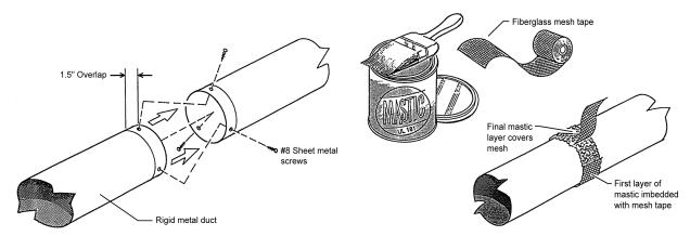
Figure 4-20: Sealing Metallic Ducts With Mastic and Mesh
