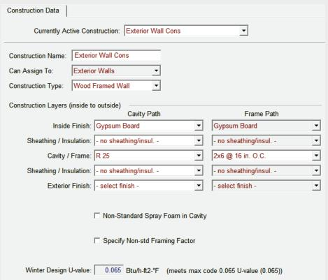
CBECC-Res Software Wall Assembly Construction showing U-0.065 Assembly
