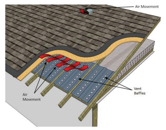
Figure 3-26: Insulation Air Baffles
