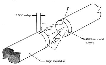
Figure 4-17: Connecting Round Metallic Ducts
