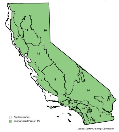
Figure 3-4: Package A, Prescriptive West-Facing Window Area Limits by Climate Zone
