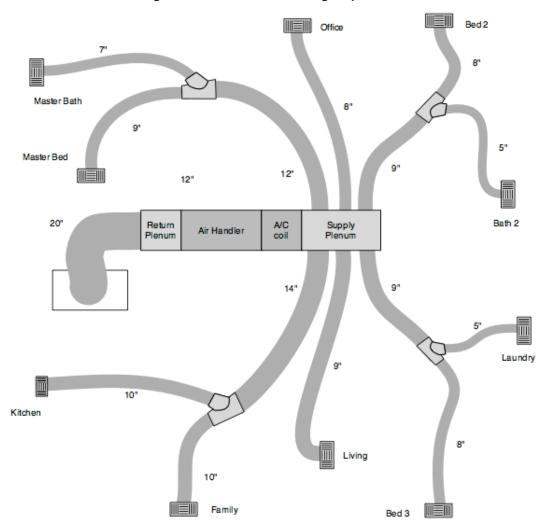
Figure 4-6: Return Duct Design Option 1
